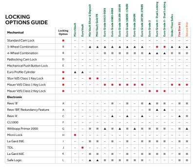
Unless otherwise stated Securikey products will be supplied with a key lock as standard. The type of lock will depend upon its position within the range. Securikey recognise that there may be a requirement to add or alter the standard locking configuration. It is for this reason we offer the following alternatives.
